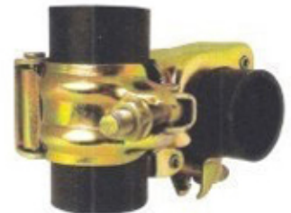
ISPC - JDC JAPANESE DOUBLE COUPLER FOR TUBE OD 48.3MM & 42.3MM (JIS : G3444 / SS-311)
